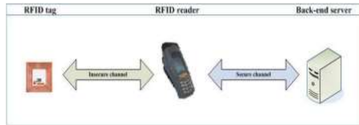
FIG 1. Architecture of an RFID authentication scheme
